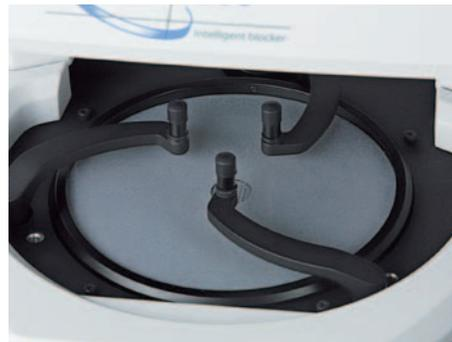
Closed position for lens blocking (multi-position lens stage is motorized)
